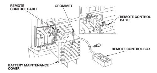
7. To avoid accidentally unplugging the remote control cable, secure the cable to the generator frame with a cable tie as shown.
