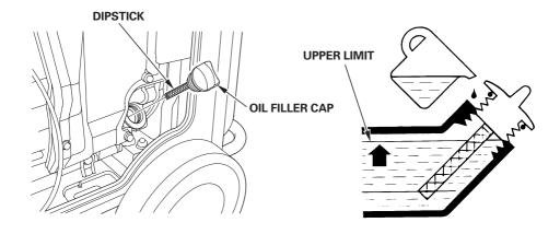
The Oil Alert system will automatically stop the engine before the oil level falls below safe limits. However, to avoid the inconvenience of an unexpected shutdown, check the oil level regularly.
