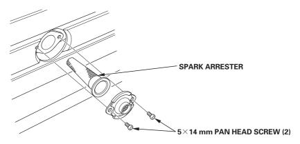
2. Use a brush to remove carbon deposits from the spark arrester screen.
