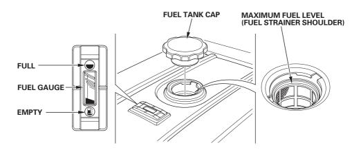
Refuel in a well-ventilated area before starting the engine. If the engine has been running, allow it to cool. Refuel carefully to avoid spilling fuel. Do not fill the fuel tank above the fuel strainer shoulder.
