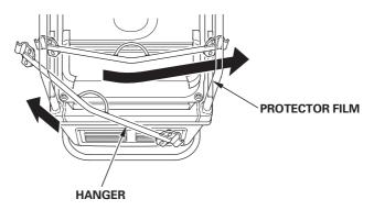
3. Slide the hanger along the frame pipe to align the center of the hanger with the recessed part on the rear side of the fuel tank. Install the hanger brackets on both ends of the hanger and tighten the 8  $\times$  16 mm flange bolts securely.
